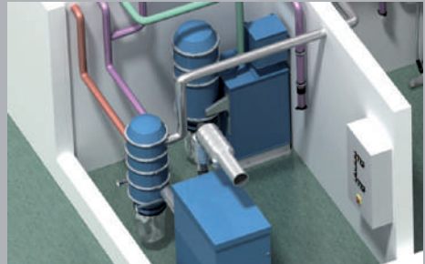
Technical central unit with dust separator, vacuum producer and controls. Designed specifically to actual requirements and always low-maintenance.
